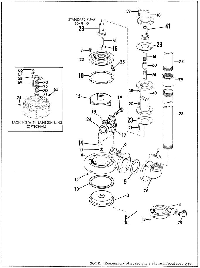
Figure 1. Model 641-642 Exploded View (Sheet 2 of 3)
