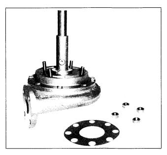
F. Nuts, support piping and gasket removed from cover.
