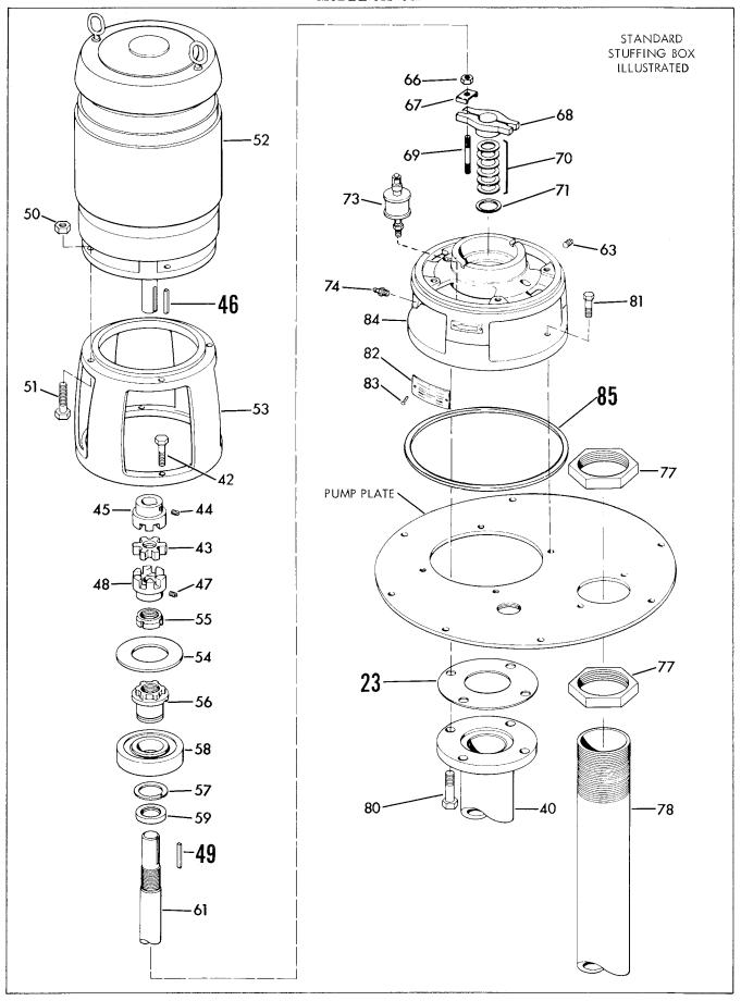
Figure 1. Model 641-642 Exploded View (Sheet 1 of 3)
