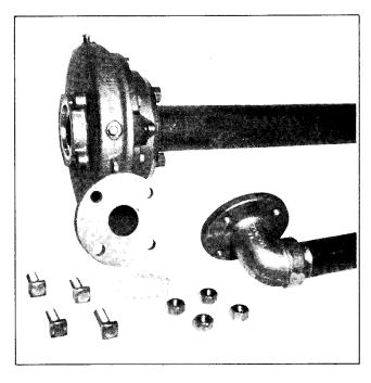
E. Nuts, capscrews and gasket removed to free discharge piping.
