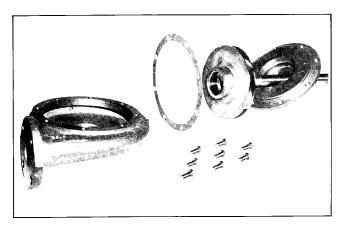
G. Capscrews, cover, casing and gasket removed to reveal impeller.
