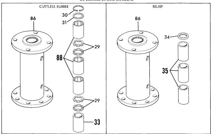
Figure 1. Model 641-642 Exploded View (Sheet 3 of 3)
